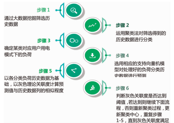
图 2 基于大数据挖掘的短期负荷预测方法流程图 Fig. 2 flow chart of short-term load forecasting method based on big data mining
